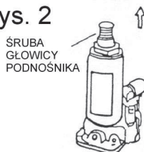
Fig. 2 Jack head screw
